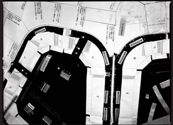
TWO OF THE SIX FORWARD-LOOKING WINDOWS—WITH PROTECTIVE PREFLIGHT WINDOW GUARDS—ON THE PILOT SIDE OF DISCOVERY. SINCE AUGUST 21, 2005, ENGINEERS HAVE REPLACED SEVEN OF THE DISCOVERY'S 10 COCKPIT WINDOWS. THE WINDOWS ARE MADE OUT OF ALUMINUM SILICATE GLASS AND FUSED SILICA GLASS, WHICH SHRINK OR EXPAND FROM HEATING ON REENTRY. MAINTAINING OPTICAL QUALITY IS ESSENTIAL FOR THE CREW DURING ASSENT AND ENTRY.
